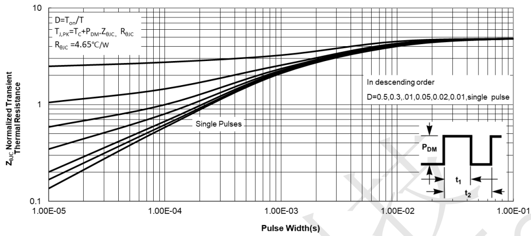
Figure 13. Maximum Effective Transient Thermal Impedance, Junction-to-Case
