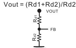
$$V_{\text{out}} = (R_{d1} + R_{d2}) / R_{d2}$$
